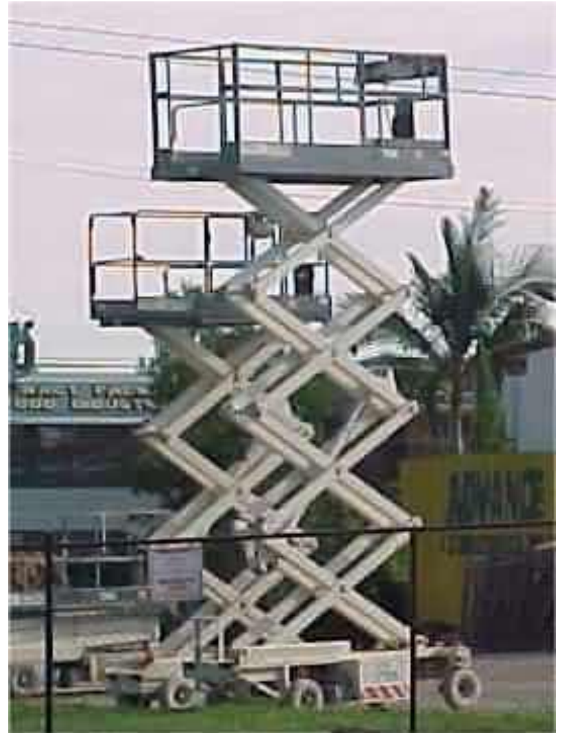
Perancah udara ( Aerial Scaffolding )
